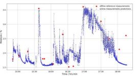
✓ PAT: Successful online monitoring of drying process/moisture content (measurement frequency ~ 1 Hz)
